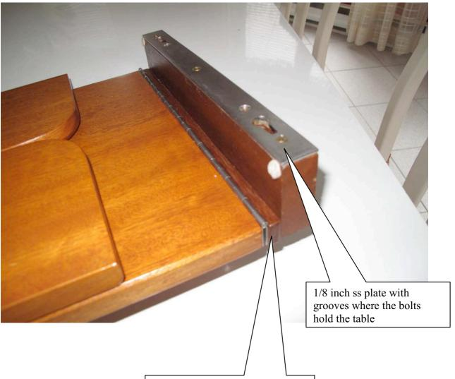
This piece of wood acts as a spacer that gives enough clearance from the stern rail that you can tilt the table vertical.
