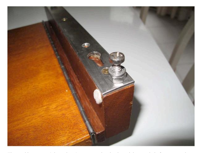
The machine screws (shown here) are screwed under the stainless steel platform across the stern. This ss platform is tapped with a ¼-20 thread. The machine screws are run into the platform just far enough to make a snug fit, then locked with the lock-washer and nut.
