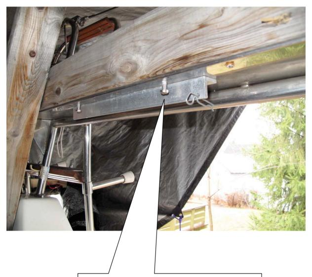
Screws under the plate. I added an aluminium angle on the back to secure the table and not put too much pressure on bolts. The pin locks the table once it is in place.
