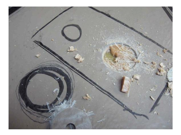
Moving on to the repair – First, I marked the area to be dried as a prelude to marking the places to drill vent holes. Lines are marked every inch to guide 3/16-inch holes, each just deep enough to pierce the layer of fibreglass.
